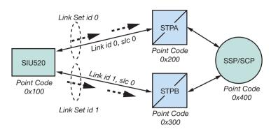
B) Traffic sent over link set 1 under failure of STP
